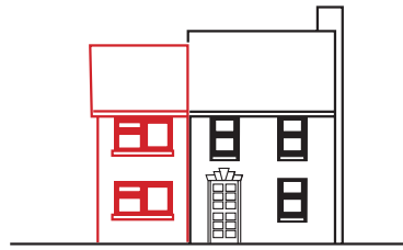
Existing character spoilt by unsympathetic windows in extension
