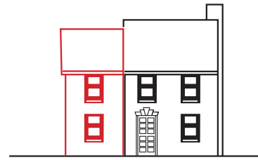
Character retained by using windows in keeping with those in the original house
