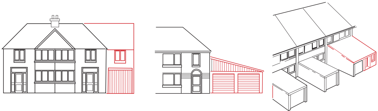
Extensions unsympathetic to the original roof form of the house
